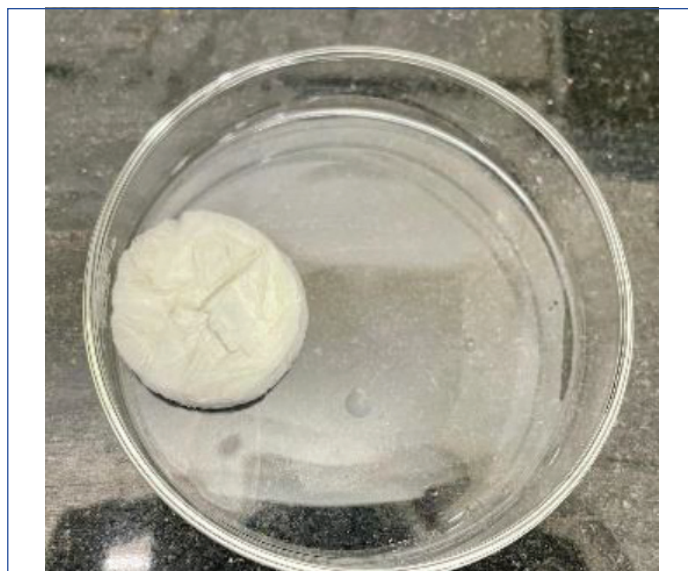
[Table/Fig-2]: Chitosan-Zinc Oxide mixture cast into sterile petri-dishes to obtain a porous CS-ZnO scaffold.
