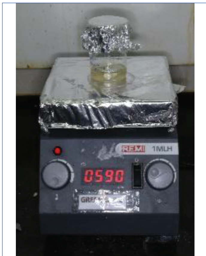
[Table/Fig-1]: Sodium hydroxide (NaOH) and Zinc Nitrate hexahydrate \{Zn(NO_3)_2 \cdot 6H_2O\} solution under continuous magnetic stirring.
