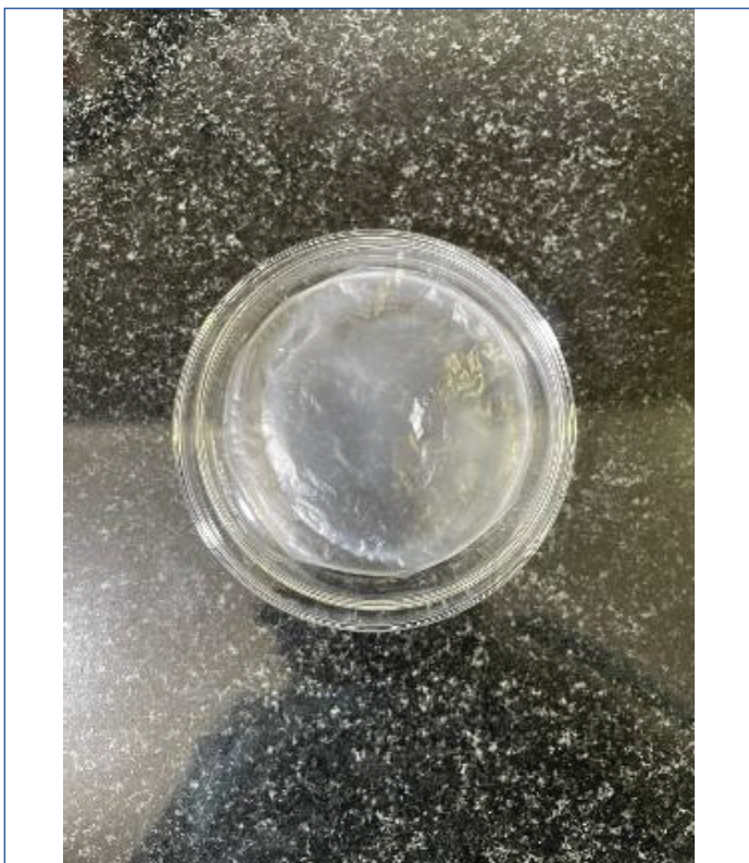
[Table/Fig-3]: Uniform PCL film after complete solvent evaporation.
